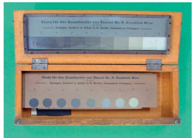
Fig. 4 Kienböck's Quantimeter used to measure the dose of X-ray radiation on display at the Museum of the Institute for the History of Medicine, Medical University Vienna.
